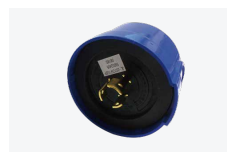
NEMA Photocell > Rated Voltage: 110-277V > Rated Loading: 1000W > Tungsten, 1800VA Ballast > Power Consumption: 1.5VA > On/Off Level: 6Lx On/50Lx Off > Related Humidity: 99%
